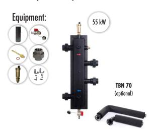
Hydraulic separator **CPN 70** is made of steel. The factory is equipped with insulation, the upper side with two connections for the temperature sensor and a vent (coupler  $\frac{1}{2}$ " F), and the lower side of the drain connection (coupler  $\frac{1}{2}$ " F). In the set they are automatic air vent  $\frac{3}{8}$ " with check valve  $\frac{1}{2}$ ", immersion sleeve for temperature sensor  $\frac{1}{2}$ ", drain valve  $\frac{1}{2}$ ", four cast-iron fittings 1" and wall brackets.
